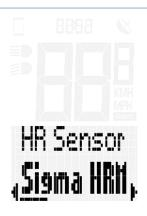
All heart rate sensors found will be shown in a list. Choose the sensor you want to connect with the EOX® REMOTE 500 using the A/C buttons and confirm the connection by pressing the B button.
