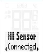
Once the connection has been established the status of the menu changes to "HR Sensor Connected".
