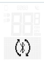
Press the B button to search for available Bluetooth heart rate sensors. The heart rate belt must be activated before starting the search.
