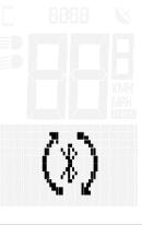
Press the **B** button to search for available Bluetooth heart rate sensors. The heart rate belt must be activated before starting the search. HR Sensor "<u>Si</u>gma HRM,
